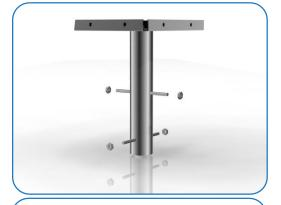
1. Using M10 nuts and 200mm bolts supplied locate through pre drilled holes and secure bolts in place to support in ground pole in concrete. (See Assembly Guide)
