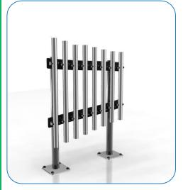
1. Carefully lay 2 x legs on a level surface and check distance between legs is equal. Line up pre drilled holes in the backboards with the holes in legs and ensure the instrument is aligned square with the legs. Fix in place using M8x40mm screws supplied (see installation guide)
