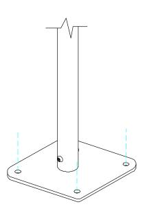
Fix Surface Plate to the ground surface **Ground Anchors Not provided**cover fixings with caps provided
