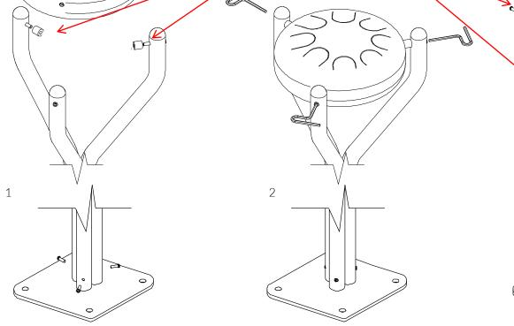
Locate the Surface fix Plate into the leg of the instrument.
